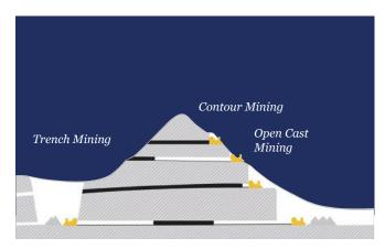
Whether you're operating a trench, open cast or contour mine, the Gainwell highwall mining system can extract coal affordably and safely.
